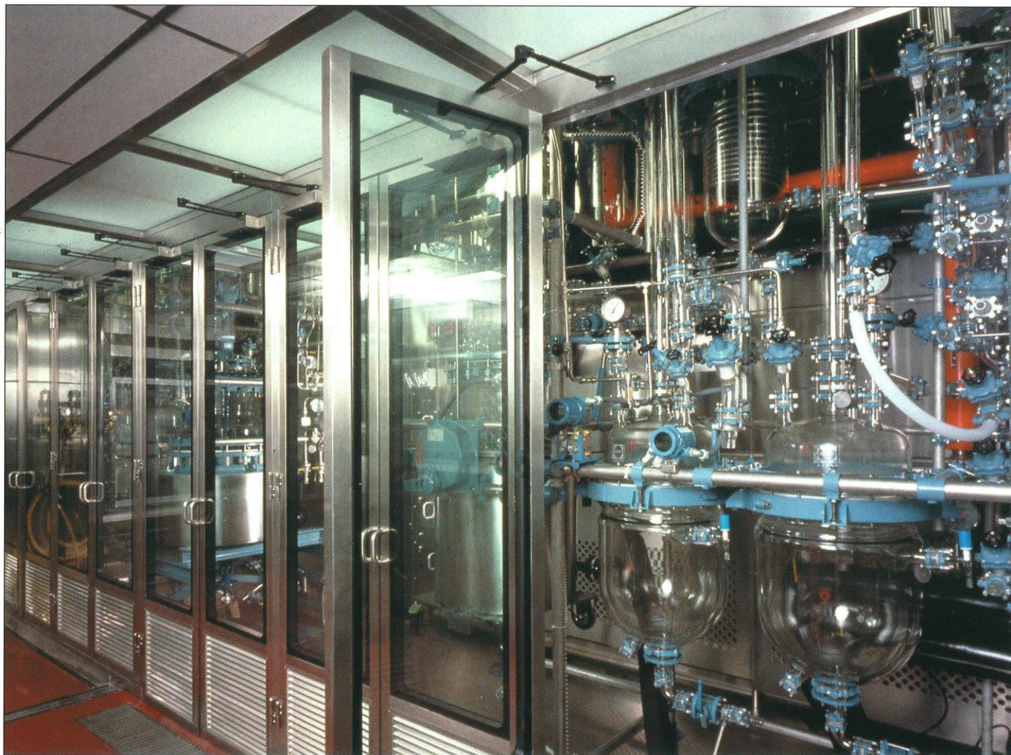
Figure 6. The Buchi systems are located entirely within downflow booth enclosures to protect the operator from exposure to dangerous solvents.
