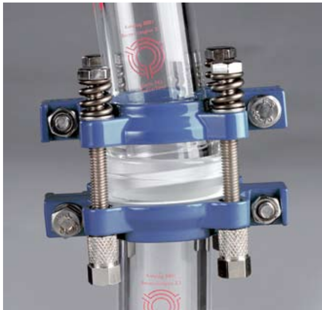
即使两个部分不是完全的对准，每个接头也都能由四颗带有弹簧的螺钉很好的固定 Assembling the join using four screws with springs gives a perfect seal, even if the two pieces are misaligned
