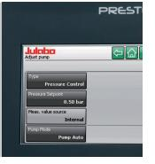
**Tip** The Ethernet interface permits full access to all operational functions of the PRESTO®.
