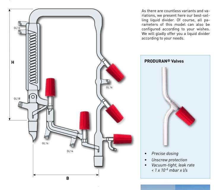
**Liquid Divider with Intensive and Intercooler, Dead Volume free** In- an outlet NS 29/32, intensive cooler 200 mm
