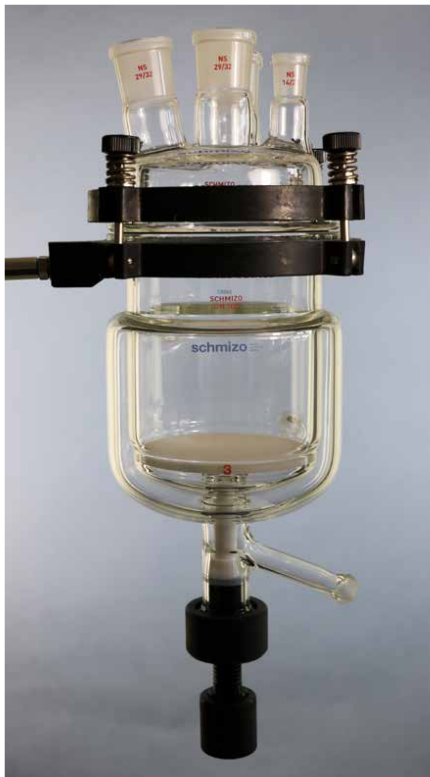
Jacketed reactor with fused-in glass filter plate P3
